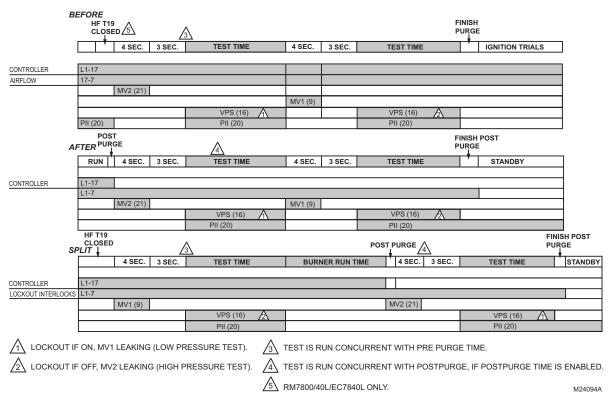
Fig. 5. RM7800L/40G,L and EC7840L Relay Module operation, Valve Proving test options.
