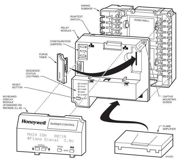
Fig. 8. RM7800L/40L, EC7840L Relay Module exploded view.
