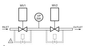
CAUTION: VALVE ENERGIZING TIMING IS BASED ON HONEYWELL VALVE OPENING TIMES OF 13 SECONDS MAXIMUM. - FOR VALVES WITH TIMINGS GREATER THAN 13 SECONDS OR THOSE THAT DO NOT OPEN THE ACTIVE VALVE WITH IN THE ENERGIZED TIME, A BYPASS SSOV RATED SOLENOID VALVE (1/4", 120 VAC) IS REQUIRED TO OBTAIN THE PROPER TEST PRESSURES. - THE BYPASS VALVE WILL BE WIRED IN PARALLEL TO THE VALVE IT IS BYPASSING (TERMINAL 9 FOR MV1 OR TERMINAL 21 FOR MV2).
