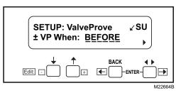
Fig. 12. SETUP: Valve Prove screen.
