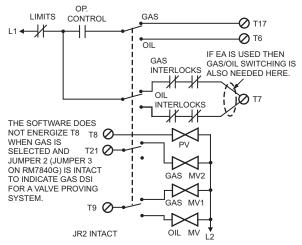
R. VALVE PROVING: GAS DSI, OIL 10 SECOND MFEP
