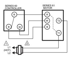
AND OVERLOAD PROVIDE DISCONNECT MEANS AND OVERLOAD PROTECTION AS REQUIRED.
