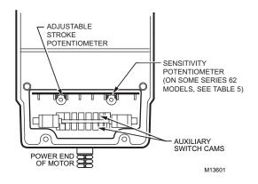
Fig. 12. Stroke adjustments setup.
