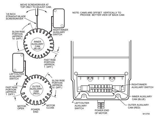
Fig. 14. Auxiliary switch adjustment.
