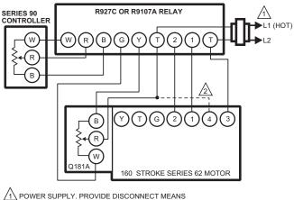
AD POWER SUPPLY. PROVIDE DISCONNECT MEANS AND OVERLOAD PROTECTION AS REQUIRED. ∧
