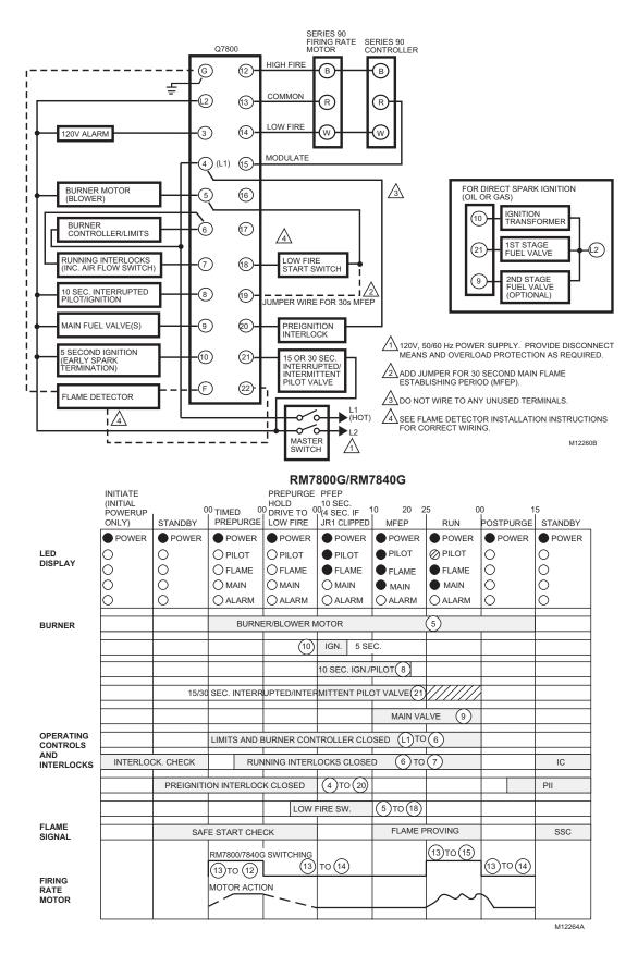
Fig. 3. Wiring subbase and sequence for RM7800G/RM7840G.
