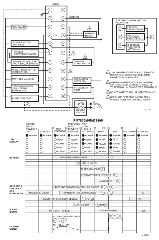
Fig. 4. Wiring subbase and sequence for RM7800M/RM7840M.
