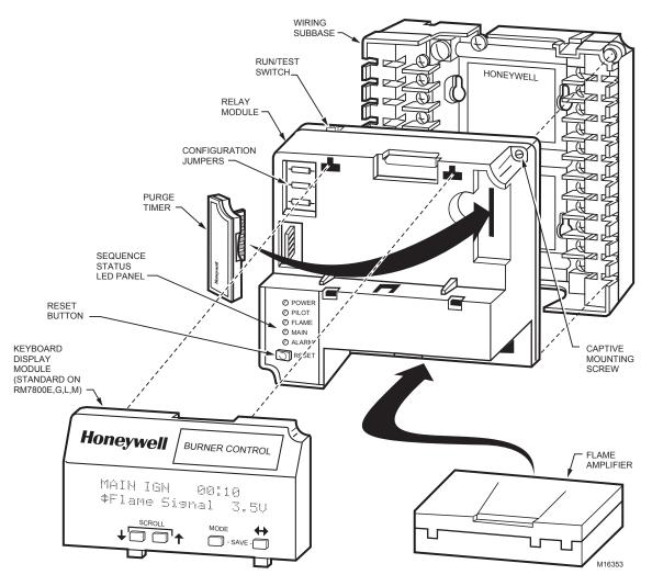
Fig. 5. RM7800/RM7840 Relay Module exploded view.
