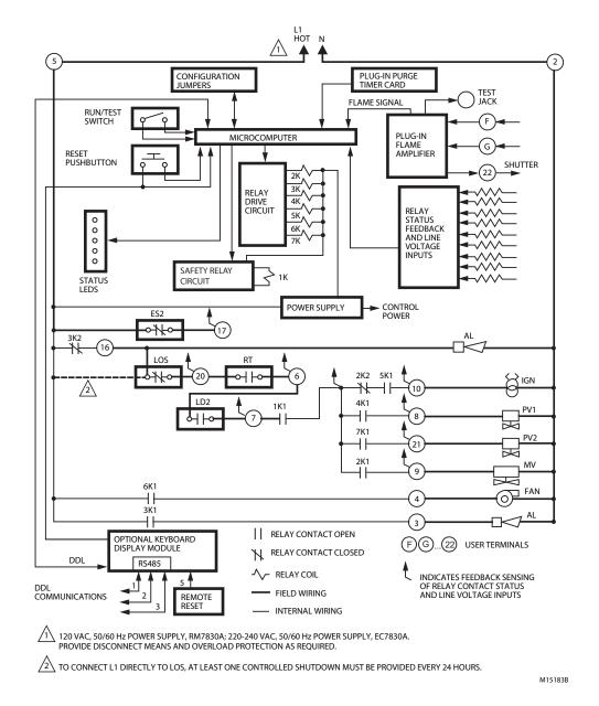
Fig. 1. Internal block diagram of EC/RM7830A (see Fig. 3 for detailed wiring instructions).
