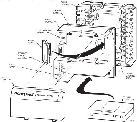
Fig. 5. EC/RM7830A and EC/RM7850A Relay Modules exploded view.
