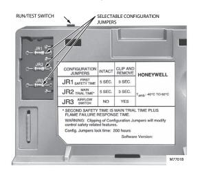
Fig. 6. Selectable site-configurable jumpers.
