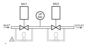
CAUTION: VALVE ENERGIZING TIMING IS BASED ON VALVE OPENING
