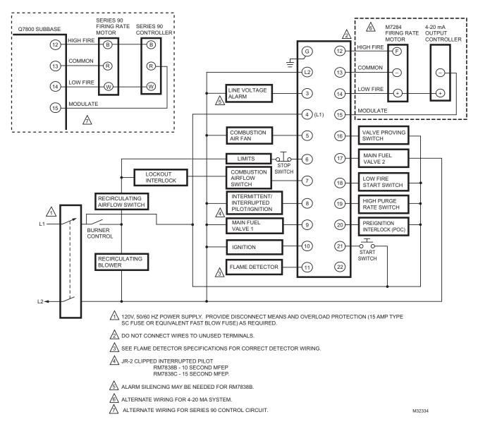
Fig. 3. Wiring subbase for RM7838B,C.
