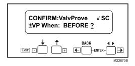
Fig. 15. Confirmation Acknowledgement screen. (The Valve Proving Test location is shown.)
