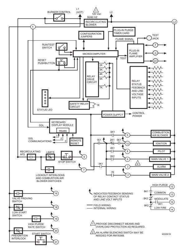
Fig. 2. Internal block diagram of RM7838B,C.
