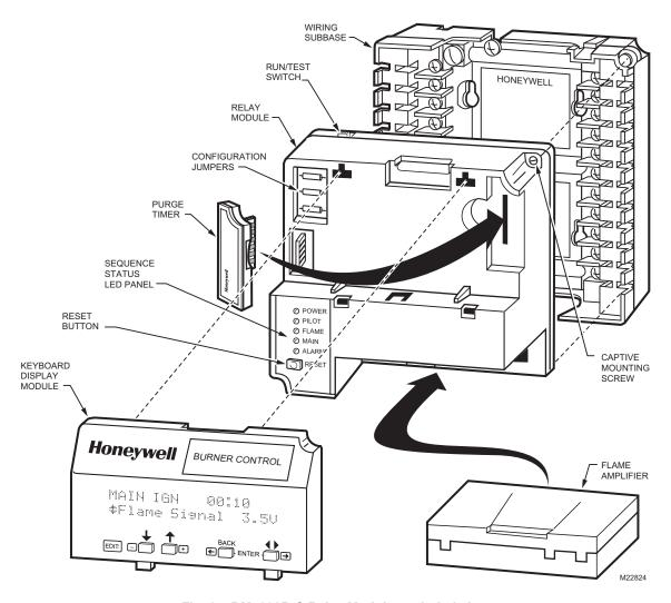
Fig. 24. RM7838B,C Relay Module exploded view.
