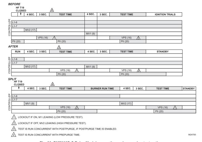
Fig. 23. RM7838B,C Relay Module operation, valve proving test options.
