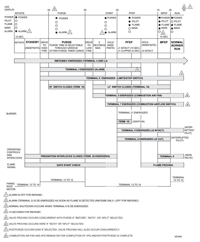
Fig. 25. RM7838B,C Relay Module operation.
